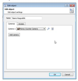
Adding a camera to an object will mean that, whenever there is an event on that object, the recording from that camera will be related to the time and date of the object event, in the Integration database.
